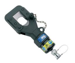
Hydraulic cutting head complete with quick automatic coupler for connection to a hydraulic pump with a working pressure of 700 bar max
